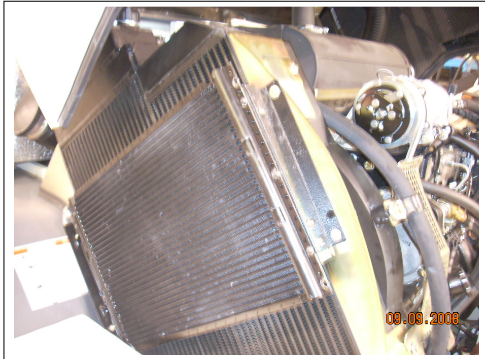
Condenser mounted in place.
