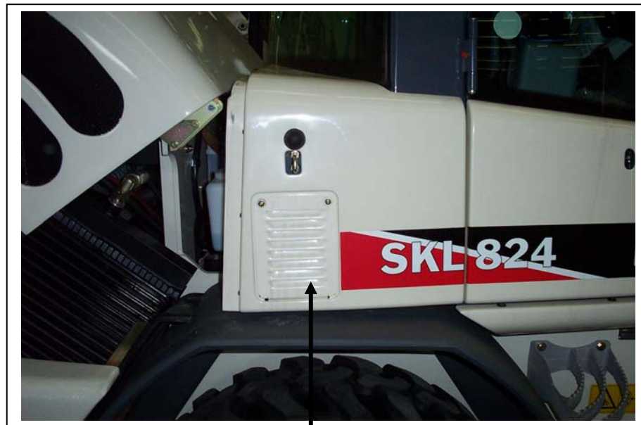
Air intake panel back in place.
